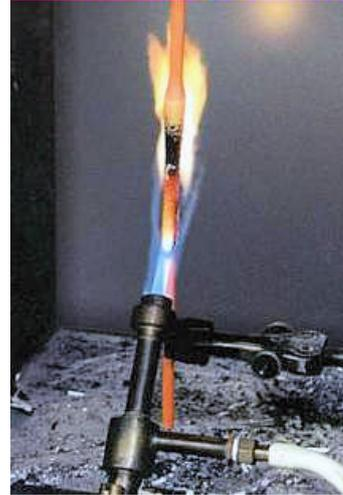
IEC 60332-3 is the test method that properly simulates cables installed in real-life sites, where tenth or even hundreds of cables are packed together.
