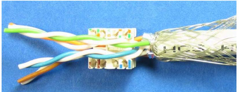
**4** Insert the wires into the correct colored slots.
