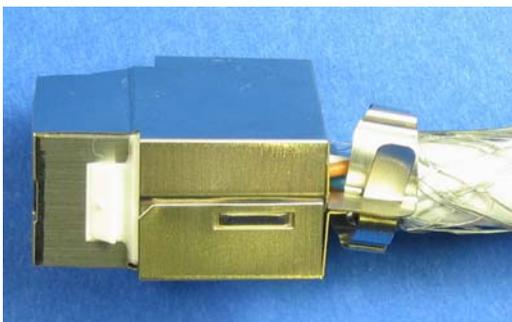
**12** Pull the grounding belts with a suitable pliers and fold them.
