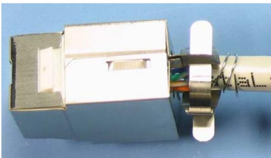
**12** Pull the grounding belts with a suitable pliers and fold them.
