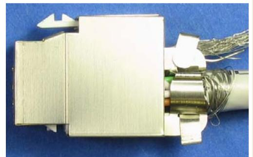
Note: Avoid damaging the cable when using the pliers and make sure the braid shield is in good contact with the keystone jack shield.
