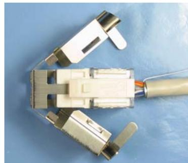
**10** Wrap the drain-wire around the cable and close the metal shield.
