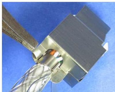
**13** Wrap the shield and press tightly both grounding belts.
