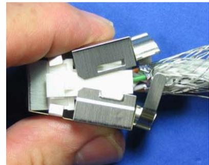
**11** Make sure the two grounding belts are inserted into the two slots.
