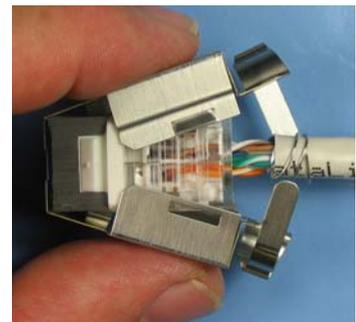
**11** Make sure the two grounding belts are inserted into the two slots.
