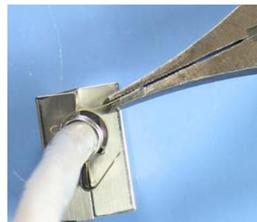
**13** Wrap the ground wire and press tightly both grounding belts.
