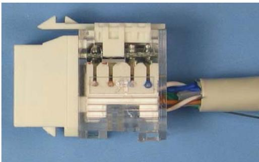
**9** Slide the metal shield over the jack. Note the correct orientation.
