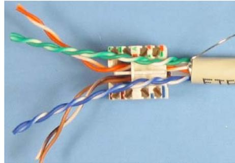
**4** Insert the wires into the correct colored slots.
