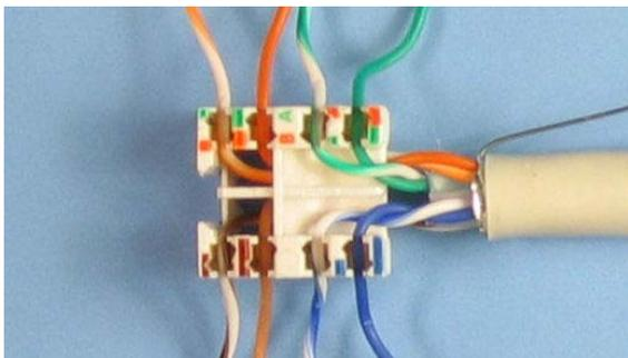
**5** Cut the wires flush with a sharp tool.
