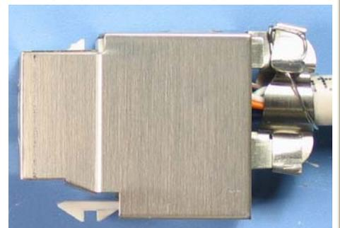
Note: Avoid damaging the cable when using the pliers and make sure the drain wire is in good contact with the keystone jack shield.
