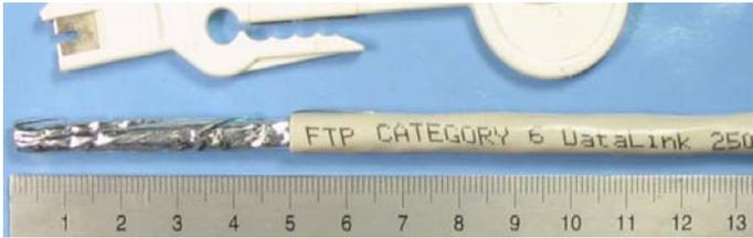
**2** Carefully remove the foil shield.
