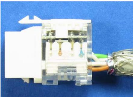
**9** Slide the metal shield over the jack. Note the correct orientation.
