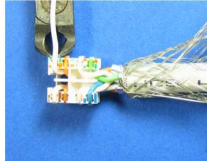
**6** Slide the wiring block into the the jack housing with the colored side down and push gently with your thumb. Note the guide and the IDC contacts.
