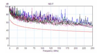
Another important benefit provided by Reelex II<sup>TM</sup> box packaging is the ability to test NEXT loss and Return Loss in each and every box shipped. This final testing, which is part of the famous HCS Double-Safe<sup>TM</sup> Program, cannot be done when cables are packed in reels or in reel-in-box, as the parallel layers of cables provides incorrect test results.
