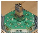
**HCS DataLink 500A** Augmented Category 6 unshielded and fully shielded Keystone Jacks, HCS P/N <u>J6A-00813</u> and <u>J6A-00823</u>, were specially engineered to perform well beyond Category 6A standards in all transmission parameters, maintaining a minimum of 3dB NEXT margin up to 500MHz in all combinations, even in short permanent links (15m min. length, as specified in ISO/IEC-11801).
