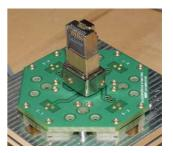
**HCS DataLink 500A** Augmented Category 6 unshielded and fully shielded Keystone Jacks, HCS P/N <u>J6A-00813</u> and <u>J6A-00823</u>, were specially engineered to perform well beyond Category 6A standards in all transmission parameters, maintaining a minimum of 3dB NEXT margin up to 500MHz in all combinations, even in short permanent links (15m min. length, as specified in ISO/IEC-11801).
