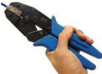
6. Carefully insert the assembly which you have just completed into the modular crimping tool. When crimping the connector make sure you use the full stroke of the crimp tool so that the contacts properly "bite" into the conductors. After you have completed the crimp take time to look at the connector and make sure all the pins were crimped and that they made good contact with the conductors.
